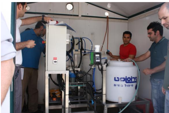
ED Pilot plant at GAT BWRO desalination plant of Mekorot
