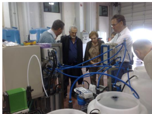
ED Pilot plant at GAT BWRO desalination plant of Mekorot
