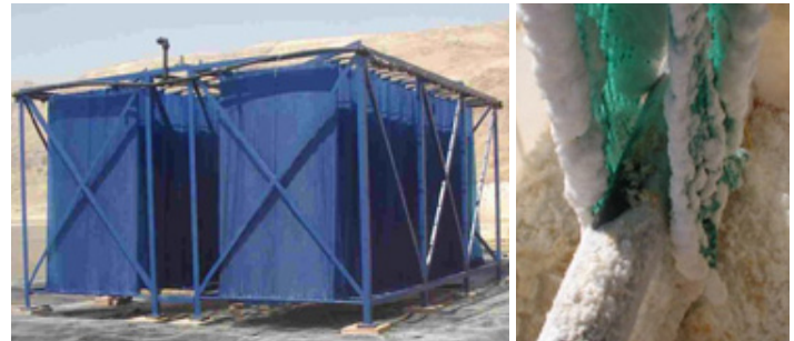
NaCl Salt Cake on Plastic Elements
